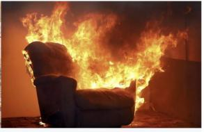
A chair burning in an open container without a sprinkler system shows the dangers of not having a sprinkler. In an enclosed room poisonous gas and heat would rapidly build up. The climbing temperature could cause a flashover where every combustible surface exposed to the fire's heat bursts into flame. (Steve Kuchera / skuchera@duluthnews.com)
